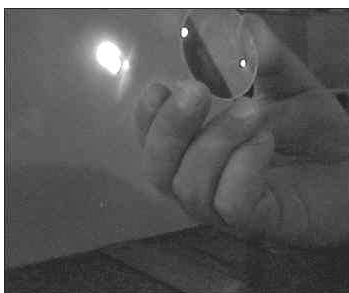
Figure 3 - Finding the focal length (20cm lens) with a ruler and light source – make the light circle as small as possible
