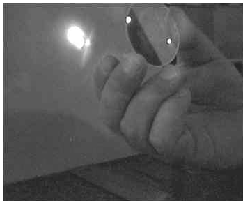
Figure 2 – A positive lens made of glass – one that refracts light
