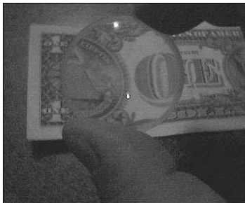
Figure 11 - Magnification where a positive glass lens is held less than 1 focal length from an object – a virtual erect image is created
