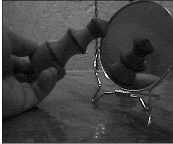
Figure 10 – A single positive reflecting lens mirror – a chess piece held close to the mirror is magnified, but the image is virtual
