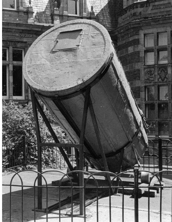
Figure 26 – The mirror housing of Herschel’s 40 foot telescope (courtesy of M. Tabb, The William Herschel Society)
