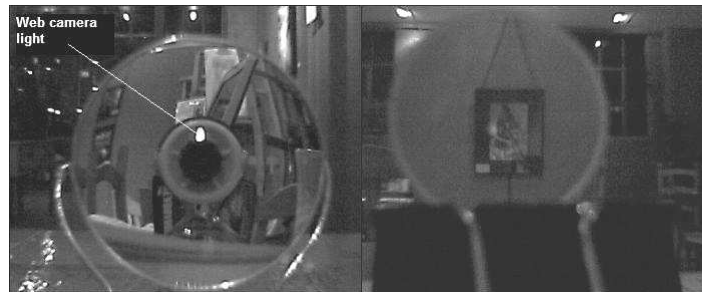
Figure 14 – A single positive reflecting mirror (left) near one focal length and a positive refracting lens (right) at less than one focal length looking at a distant object more than one focal length away
