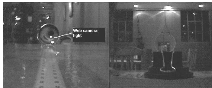
Figure 17 – A single positive reflecting mirror (left) moving past two focal lengths and a positive refracting lens (right) moving past one focal length – the image inverts
